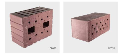
The heavy clay bricks 3DF and 2DF 2000, load-bearing, are heavy extruded clay bricks of application class II for clad, weather-protected exterior masonry and any type of interior masonry, with a hole fraction  $\leq$  15%. They are suitable for load-bearing clay brick masonry and meet the compressive strength class 5 according to DIN 18945. The 3DF format allows for economical single-layer bricklaying of walls 17,5 and 24 cm thick. ClayTec clay mortar is suitable as mortar.
