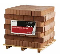
Heavyweight extruded clay blocks of application class II, for drywall construction and interior masonry. The clay block 1800 DF is a solid block. Because of its low weight, it is usually used for ceiling infills, supports and stacked layers in drywall construction work. Clay block 1800 NF is also used for masonry work. Clay masonry mortar is suitable as a mortar.
