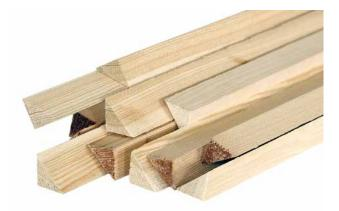
**Larch or oak wood battens** for connecting between masonry and timber-frame beams. The cross section is sufficiently flexible and adaptable even for old and irregular beams. The height corresponds to the thickness of the clay mortar joint at the end of the open space. The larch wood is stable, durable and easily nailed. Triangular battens made of oak are very suitable for half-timbered houses made of oak.
