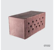
The heavy clay bricks 3DF and 2DF 2000, load-bearing, are heavy extruded clay bricks of application class II for clad, weather-protected exterior masonry and any type of interior masonry, with a hole fraction ≤ 15%. They are suitable for load-bearing clay brick masonry and meet the compressive strength class 5 according to DIN 18945. The 3DF format allows for economical single-layer bricklaying of walls 17.5 and 24 cm thick. ClayTec clay mortar is suitable as mortar.
