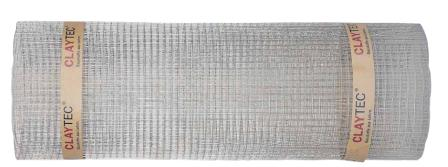
Plaster lath for severely weathered timber-frame infill sections. Stainless steel mesh plaster lath is rust free and specially formed. The recesses allow the necessary distance to be kept from the plaster base. It is held in place using facade fixing screws. With unusually weathered and exposed timber-frame constructions, it offers additional security for ensuring that lime render stays attached.
