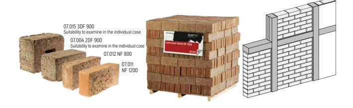
Lightweight mould-made clay block of application class Ia (= approved for timber-frame masonry work) in format NF. The composition and manufacturing technique make it very resistant to moisture and frost. The historical normal format (NF) lies well in the hand, the size is just right for timber-frame construction. The 1200 NF clay block can be knocked and cut into shape very easily. Lightweight clay masonry mortar is an ideal mortar for plastering with coarse lime basecoat render with hair.
